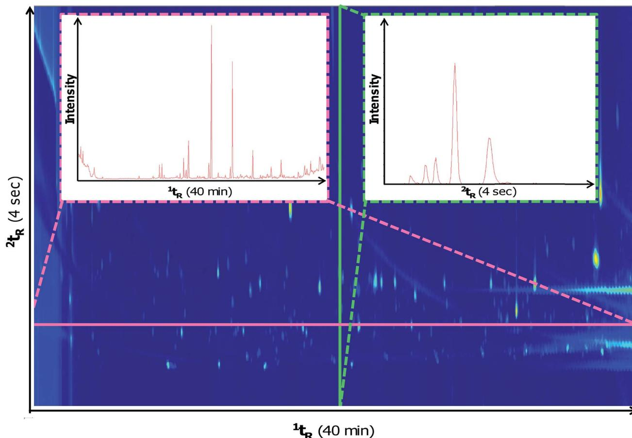
Fig. 1 Total ion current (TIC) contour plot of a decomposition soil VOC sample. The x-axis represents first dimension retention time ( ${}^1t_R$ ) and the y-axis represents second dimension retention time ( ${}^2t_R$ ). Projected slices of the contour plot are displayed for the <sup>1</sup>D (pink) and <sup>2</sup>D (green).
