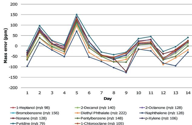
Fig. 3 Mass errors (in ppm) of selected compounds based on the measured  $m/z$  in comparison to the accurate  $m/z$  over a two week period.
