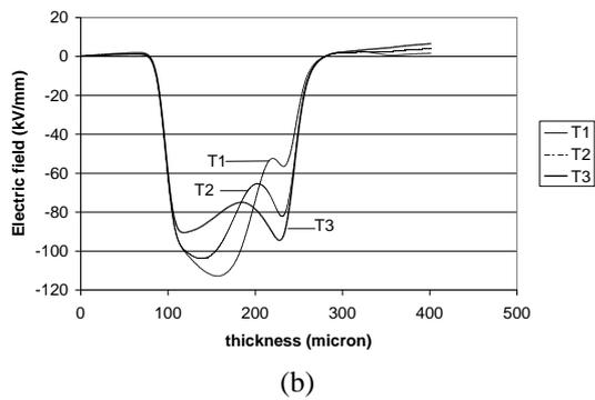
Fig. 5(a) and (b) shows space charge and the internal electric field profiles respectively when the applied electric field was reduced to 90kV/mm. The duration of electrical stress was for 0.5 hour. Time T1 is at 81s, T2 at 810s and T3 at 1620s.
