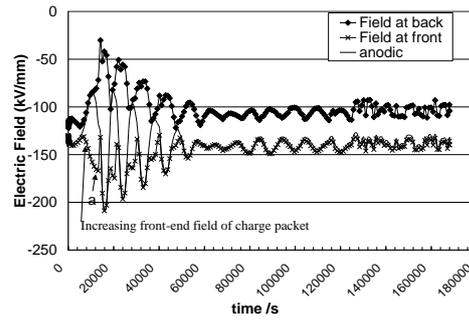
Fig. 3 Temporal change of local internal electric fields at the front, at the rear of the charge packets together with the anodic field. Applied electric field at 120kV/mm.
