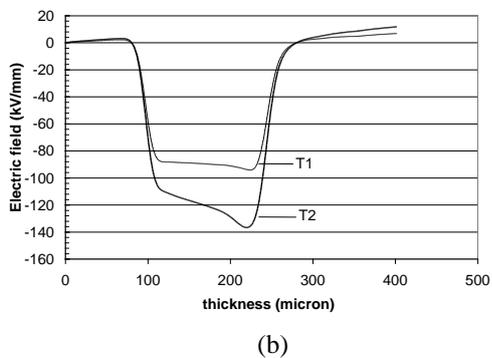
Fig. 6(a) and (b) shows space charge and the internal electric field profiles respectively when the applied electric field was re-increased to 90kV/mm for 1 hour and later to 120kV/mm for the last 1 hour.
