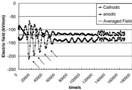
Fig. 2 Comparison of the temporal change of local internal electric fields at the anode and cathode sides. Average applied electric field at 120kV/mm
