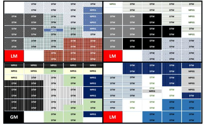
Fig. 2: Application mapping in a 10x10 NoC-based platform.
